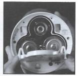
3. Insert 3- D batteries (not included). Follow diagram on battery case for proper orientation.
